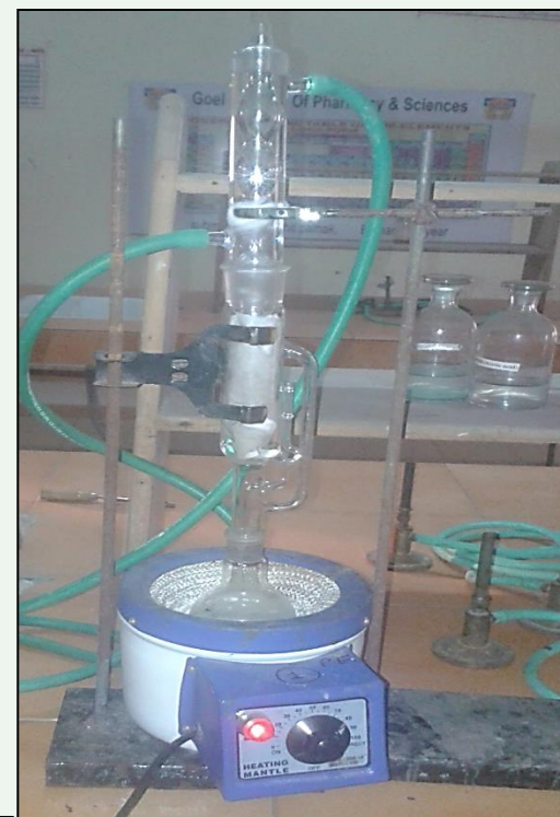
Extraction in Soxhlet apparatus
