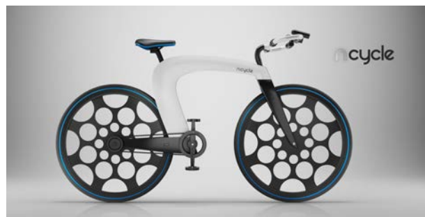
E-bike of the future: nCycle designed by Skyrill and Marin Myftiu: The novel bicycle frame is constructed from a pair of side panels, which conceal a battery, storage compartment, an optional folding mechanism, and integrated safety and security features. nCycle is intended to represent an electric conveyance that is "cheaper, sturdier, more flexible, easier to build and maintain."
